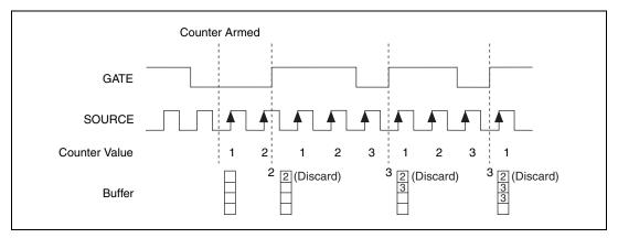
Figure 7-9. Buffered Period Measurement
